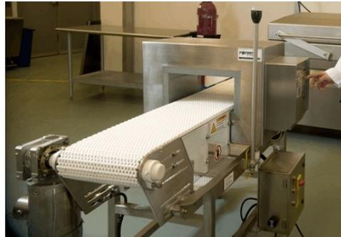
FTC's newly acquired metal detector uses the latest digital signal processing technology to detect and reject ferrous and non-ferrous metals including stainless steel. It is ruggedly built to withstand the harshest pilot plant applications, and is completely waterproof.
