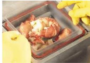
Modified Atmospheric Packaging (MAP) involves changing the gas composition in packaging to a mixture of the manufacturer's choice. The gas mixture used depends on the food product being packaged and is typically composed of nitrogen, oxygen and/or carbon dioxide. This is used to slow down the growth of microorganisms and the rate of chemical deterioration in various food products.
