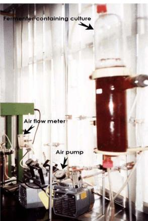
Traditionally, fermentors were designed primarily with mechanical agitation and heat exchangers. The rate of oxygen transfer depended on the interfacial areas generated by agitation, and therefore on power input to the fermentor. Studies further indicated that the total power consumption, including stirring and air compression, was about 2 kWh/kg dry cells.
