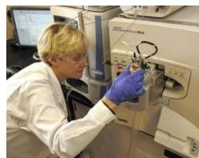
The Surveyor Liquid Chromatography system with Finnigan LCQ Advantage MAX and photodiode array detector is a powerful analytical tool in use in the FTC Natural Products Extraction Lab where biochemistry studies are performed on natural bioactive compounds for nutraceutical and pharmaceutical products.
