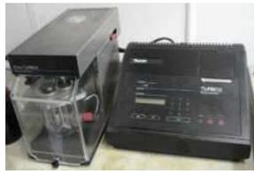
Volumetric Karl Fischer Water Titration is a widely-used analytical method for quantifying water in a variety of sample types. The fundamental principle behind this method is based on a reaction which occurs between iodine and sulfur dioxide in an aqueous medium. The amount of water this titration can detect is very small, as little as 10 ppm. There are sample conditions which are important for accuracy while performing a Karl Fischer
