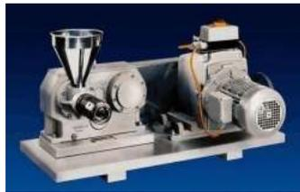
The Komet D85-1G is a versatile cold press oil extractor purchased by the Food Technology Centre to produce vegetable oils for our clients' research wherein all the vital natural components are preserved. The pilot plant-scale expeller works on a gentle mechanical screw press principle which keeps the temperature cool at less than 49°C. Virtually all oil-bearing seeds, nuts, and kernels can be pressed.
