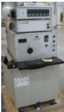
Carl Wilhelm Brabender developed the first recording torque rheometer, called a Farinograph, over 60 years ago to measure the consistency of dough in flour mixing. Since the introduction of this invention, the recording torque rheometer has evolved substantially, but the fundamental principals behind its operation have remained virtually unchanged.
