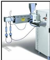
A wide range of attachments can be used with the PL 2000, and FTC presently has a 3/4" single screw extruder attachment. Currently we are evaluating the potential of this unit to produce feed materials for research purposes, but it has a very broad range of potential applications in the food industry. Contact Ed Charter, Food Science Manager, by telephone at (902) 368-5912 or by email at [eacharter@gov.pe.ca](mailto:eacharter@gov.pe.ca), if you would like further information.
