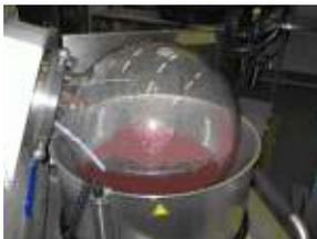
This 20 litre rotary evaporation device located at FTC increases the evaporation rate of solvents by controlling the temperature, increasing the surface area by rotating, and decreasing the pressure by vacuum.
