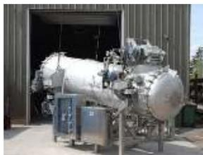
[Charlottetown Metal Products](#) has developed a patented continuous flow high pressure cooker/processor. This processor has recently been tested for different applications in the Food Technology Centre's pilot facilities. CMP has revolutionized cooker design by providing reliable processing control, continuous product flow and maximum energy efficiency.
