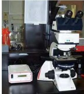
The microbiology lab has recently obtained a fluorescence microscope. This enables the use of specific antibody-labelled stains and helps improve the sensitivity and specificity in the identification of disease-causing microorganisms in food. This further enhances the ability of the lab to improve the services to its clients and to pursue research of strategic importance to food safety.
