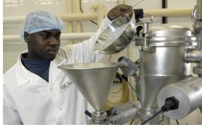
The Stephan Mixer is also equipped with a condensate collector for condensing vapour which escapes from the bowl during processing. We can recover valuable aromas and flavours to add back to the product by this feature.
