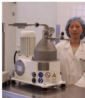
The Centre recently purchased a **GEA Westphalia Separator**, Model MTC 3-03-107, high-speed centrifugal separator with solid-wall disk-type bowl.
