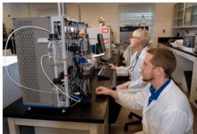
The Food Technology Centre has obtained a fully automated ÄKTA Crossflow filtration system to assist our clients in development of downstream processing. Recent advances in cross flow filtration have increased the consistency and quality of microfiltration and ultrafiltration performance which has become a technology of choice for natural product extraction in the pharmaceutical and food industries.
