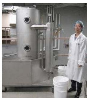
Evaporation refers to the process of heating liquid to the boiling point to remove water as vapour. Vacuum evaporation is a process that the liquid is evaporated under vacuum condition to reduce the boiling point to minimize the heat damage for heat sensitive materials.
