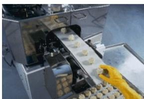
The **Rheon KN 200 Cornucopia co-extruder** is an example of one of the various items of pilot plant equipment available to FTC's clients for use in the pilot plant. This
