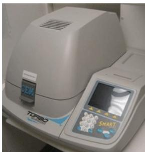
The CEM Smart System 5 is used at the FTC for rapid moisture or solids content analysis. Moisture or solids content analysis is often required when processing natural products and is used as a quality assurance test for many food products.
