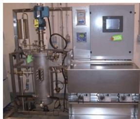
The Food Technology Centre has made a significant addition to our fermentation capacity by obtaining a 30 litre sterilizable-in-place fermenter. This new piece of equipment, designed and fabricated by Diversified Metal Engineering (DME) is intended to complement our existing R&D fermenters by allowing us to scale-up a fermentation process in a vessel that more closely represents a commercial scale fermenter.
