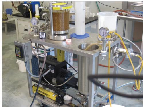
The food processing industry uses RO in the opposite configuration to remove water, and liquids such as fruit juices or maple sap can be concentrated by an RO membrane. Here, the permeate, primarily water, is discarded and the retentate is kept as concentrated juice or sap. Reverse osmosis can be used as a room temperature method of producing a concentrated product or an energy efficient way to reduce the water content of a product such as sap prior to further concentration by boiling.
